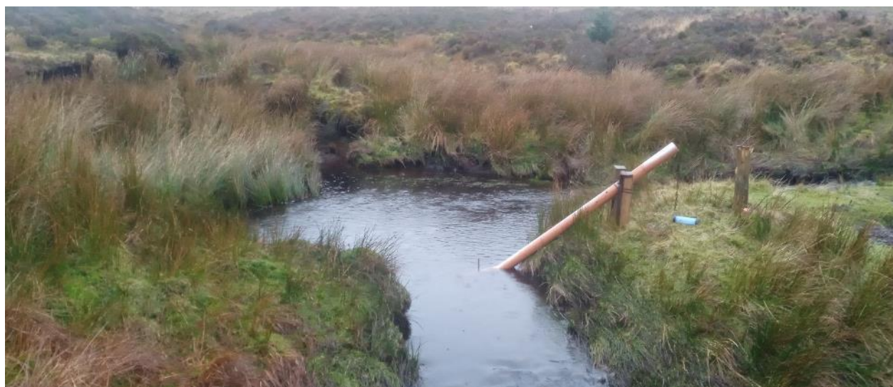
Picture 3: Frame designed to support the EXO1 Sonde at the Laggie Burn water quality monitoring site
